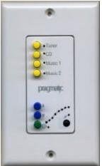
The DMS4.4<sup>TM</sup> is able to send up to four different sources to four different rooms (or zones). The system is easily expandable to add more rooms in multiple of four rooms with an expansion unit. It also easily interfaces with the door-bell/telephone interface module to provide house-wide door-bell and telephone ringing. For computer savvy users, a serial port connection allows total control of the system using a personal computer.
