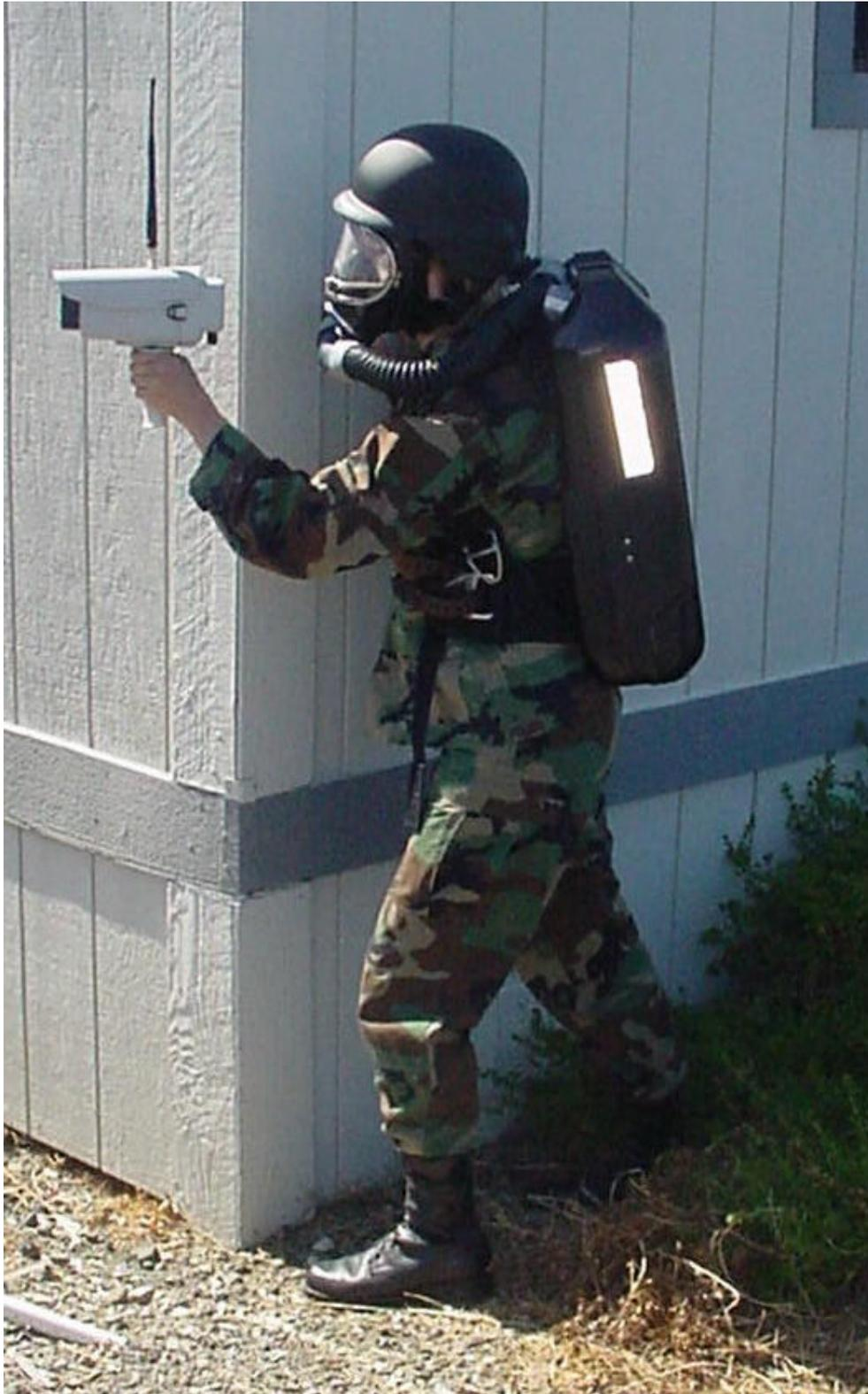
Useful in monitoring chemical, biological or other hazardous situations with a remote camera that can be mounted on a tripod. The site can be remotely monitored from a distance of more than a 1000 ft.
