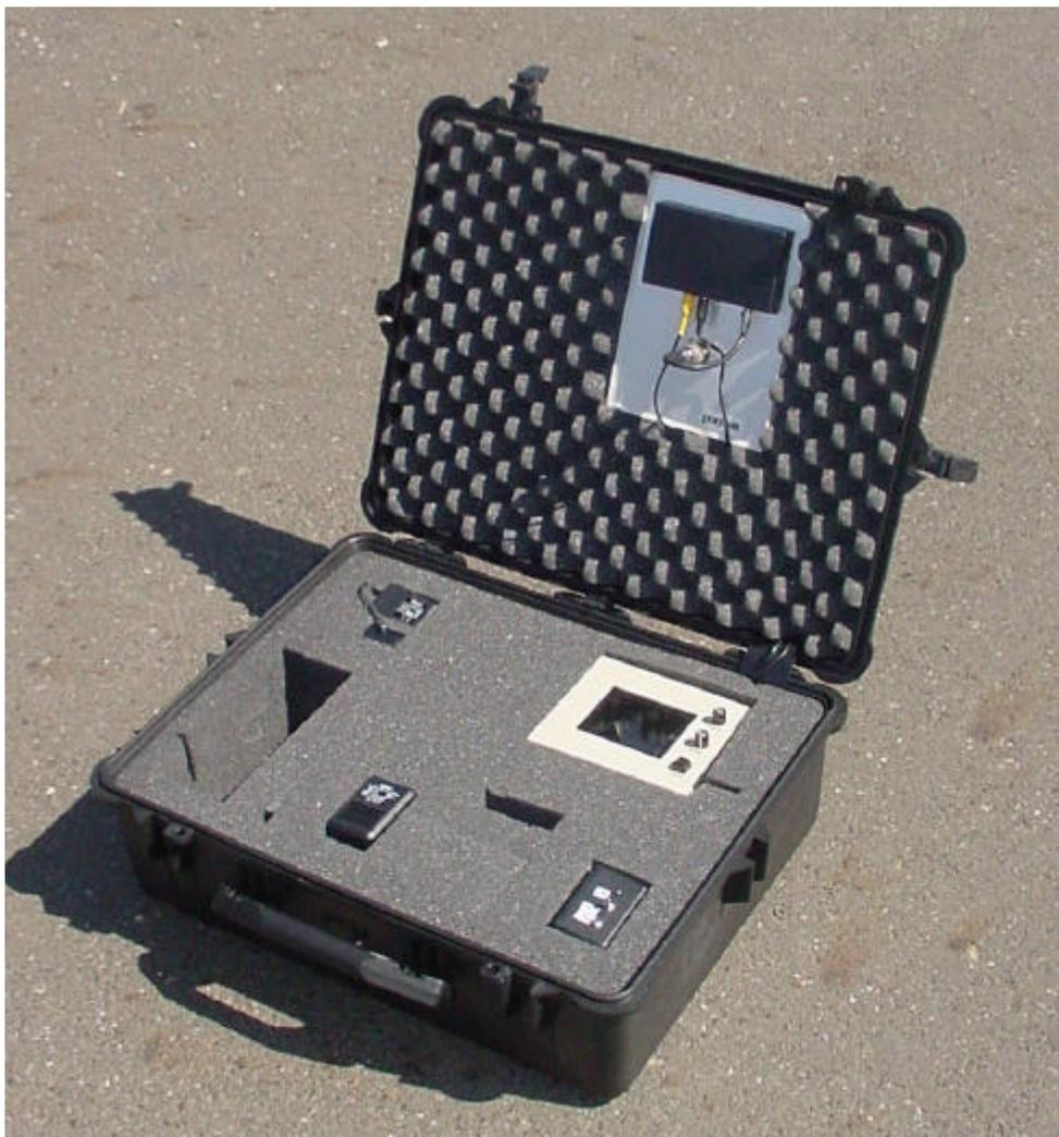
The system is fully self contained with camera, transmitter and battery pack in a single package. The receiver is housed in a rugged Pelican® case with high performance panel antenna, LCD monitor and a battery pack. Battery charger is built in the case also.
